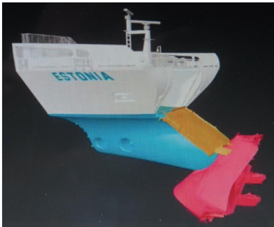
FIG. 4.5: Physical damage of the bow visor and the ramp confirming the full opening of the vessel's bow entrance at the beginning of the accident. The large dent in the front side of the visor (red) is aligned with the bulbous bow and the ramp's (yellow) underside deformations are aligned with the forepeak deck. Visor actuators are not shown.
